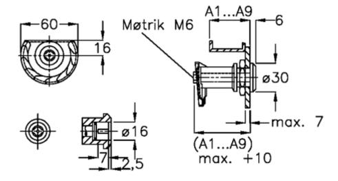
Door + frame thickness = 17-25 Measure type = A1
